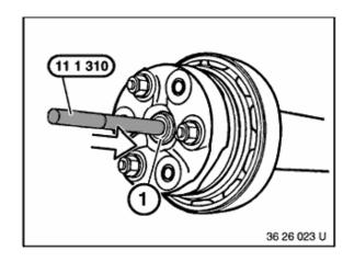
Completely fill center bore with viscous grease.
