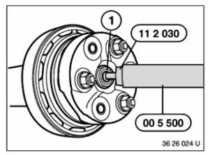
Remove grease or water from mount bore.
